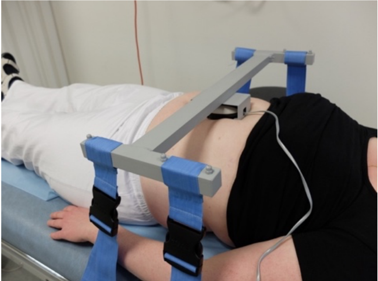
Setup for abdominal muscle strength measurement using fixated hand-held dynamometer.
