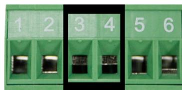
Figure 7: Fault Pin of Terminal Block.
